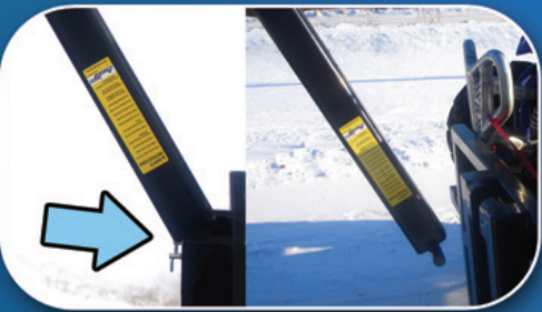
Only 2 pins for quick deck detach
