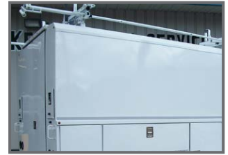
Roof-mounted single & dual pull-down assist ladder rack
