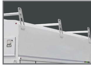
Access Ladder – Aluminum three-bar roof-mounted overhead ladder rack.
